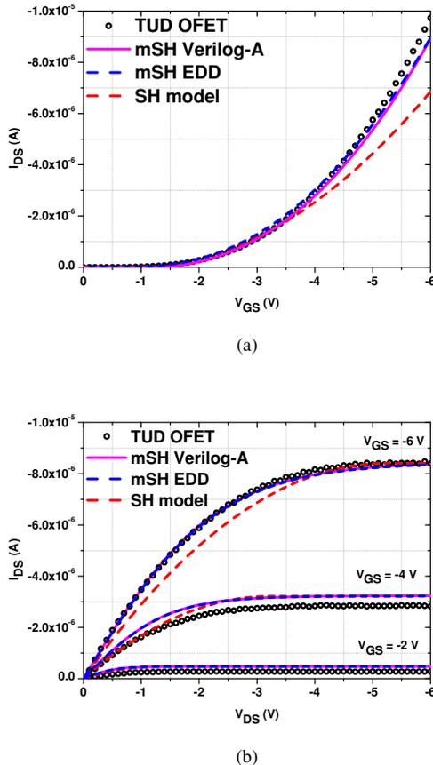
Fig. 2. Comparison of measured electrical characteristics of a TGTC OTFT with simulations employing a SH and mSH model: (a) Transfer curve for  $V_{DS} = -6$  V and (b) Output curve for  $V_{GS} = -6$  V,  $-4$  V and  $-2$  V. Note that for example at the bias point  $V_{DS} = V_{GS} = -6$  V the drain current differs for the transfer and output characteristic due to hysteresis effects.
