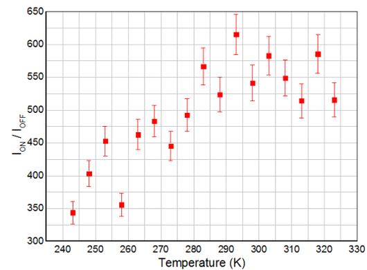
**Fig.6** -  $I_{ON}/I_{OFF}$  ratio versus Temperature curve for a n-MOS transistor.
