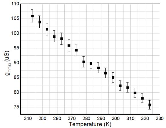
**Fig.5** – Maximum Transconductance ( $g_{mmax}$ ) versus Temperature for a  $V_{DS}=100$  mV.
