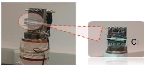
**Fig. 2** - Detail of the CD4007 Integrated Circuit positioned on the cryocooler ARS-2HW sample holder.
