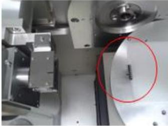
**Fig. 1** - Detail of the XRD-7000 Diffractometer at Centro Universitário FEI showing the CI placed perpendicular to the X-ray beam
