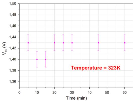
**Fig. 7** – Threshold Voltage versus Time for the unbiased device at temperature of 323 K.
