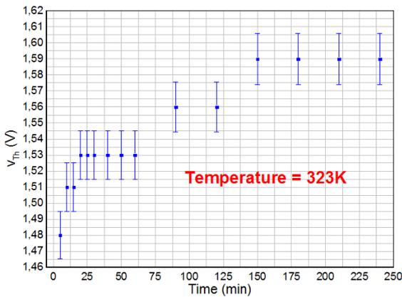
**Fig. 8** – Threshold Voltage versus Time for a constant bias of  $V_{GS}=5$  V with  $T=323$  K.
