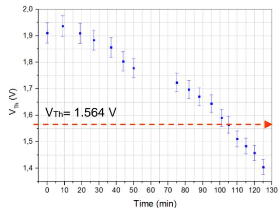
**Fig. 3** – Threshold Voltage on n-MOS transistor with a 750 krad accumulated dose and with temperature ranging from 243 up to 323 K, during more than 2 hours. Red dashed line indicates the threshold voltage after irradiation with stability in room temperature.
