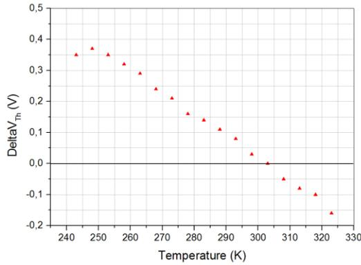
**Fig.4** – Variation of Threshold Voltage (comparison with the initial threshold voltage of  $V_{Th}=1,56V$ ) versus Temperature curve.
