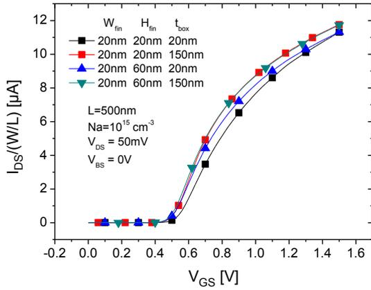
Fig. 2. (A) Normalized drain current as a function of the gate voltage for a substrate bias of 0 V.
