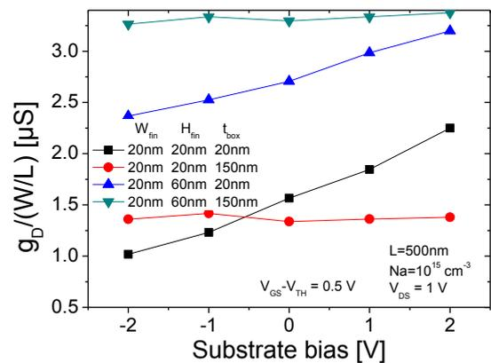
Fig. 6. (B) Normalized output conductance as a function of substrate bias varying from -2 V to 2 V for different dimensions.
