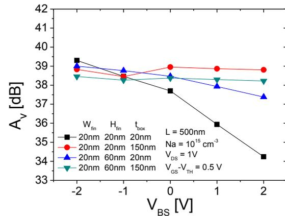
Fig. 7. (B) Gain as a function of substrate bias varying from -2 V to 2 V for different dimensions and gate voltage  $V_{GS} = 1$  V.
