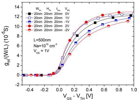
Fig. 5. (A) Normalized transconductance as a function of overdrive gate voltage for the same dimension and substrate bias varying from -2 V to 2 V.
