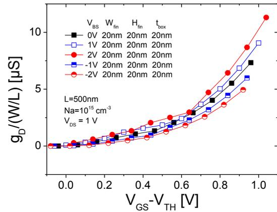
Fig. 6. (A) Normalized output conductance as a function of overdrive gate voltage for the same dimension and substrate bias varying from -2 V to 2 V.
