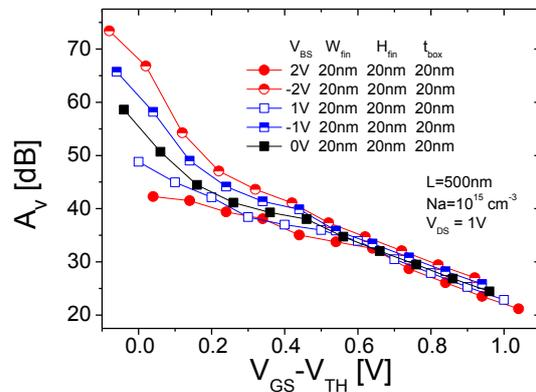
Fig. 7. (A) Gain as a function of gate voltage for the same dimension and substrate bias varying from -2 V to 2 V.
