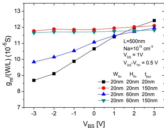
Fig. 5. (B) Normalized transconductance as a function of substrate bias varying from -3 V to 3 V for different dimensions and gate voltage  $V_{GS} = 1$  V.
