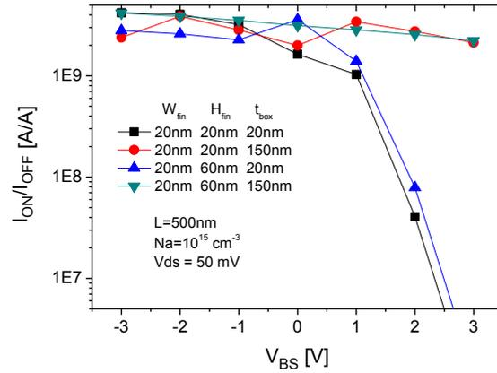
Fig. 4. Ratio of current in on state and current in off state as a function of the substrate bias.
