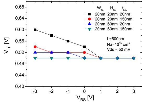
Fig. 3. Threshold voltage as a function of the substrate bias extracted from Fig. 2 for  $V_{DS} = 50$  mV.
