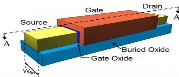
Fig. 1. Transistor SOI FinFET of tri-gate representation.
