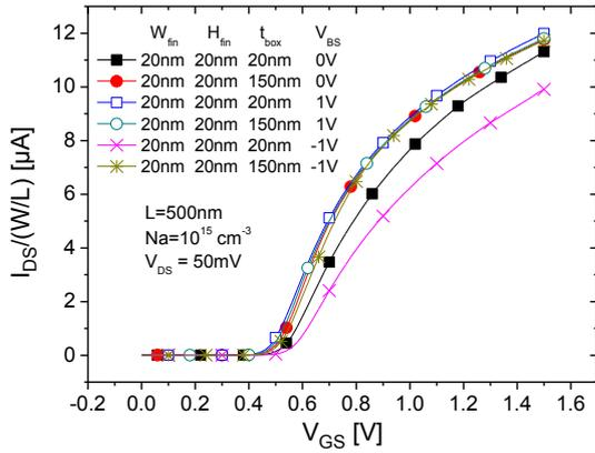
Fig. 2. (B) Normalized drain current as a function of the gate voltage for substrate bias varying from -1V to 1V and for two dimensions.
