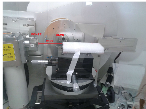
Fig. 4 – Shimadzu XRD-7000 diffractometer used to radiate the MOSFETs.
