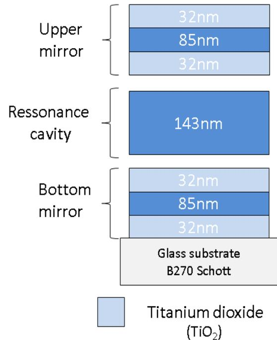
Figure 3: Structure of the blue filter centered at the wavelength of 413nm.
