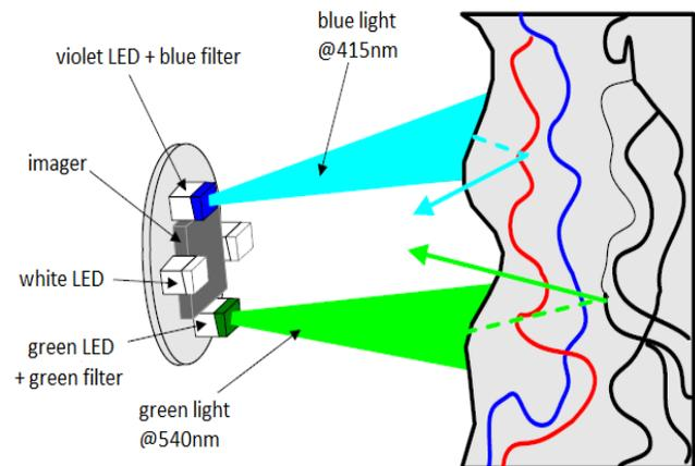
Figure 1: NBI system with LEDs along with blue and green filters and a CMOS image sensor.
