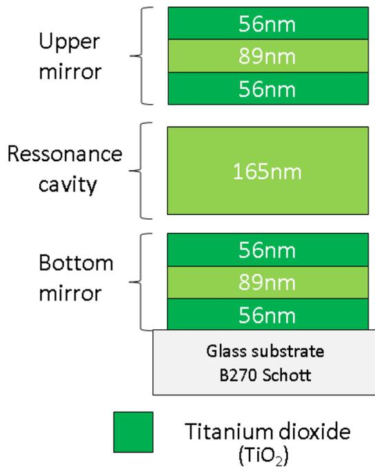
Figure 2: Structure of the green filter centered at the wavelength of 540nm.
