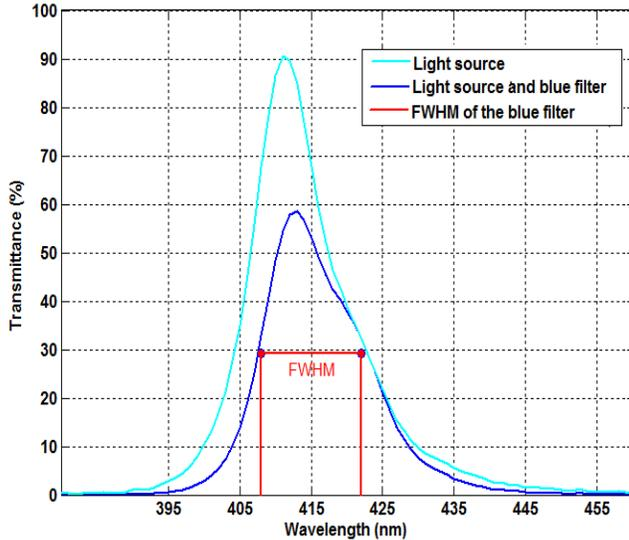
Figure 5: Simulated spectral transmittance of the blue Fabry-Perot optical filter and the light source for this filter.
