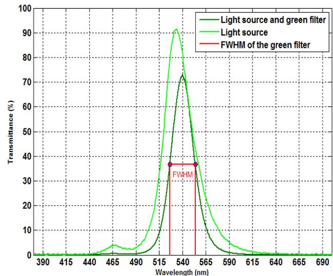
Figure 4: Simulated spectral transmittance of the green Fabry-Perot optical filter and the light source for this filter.
