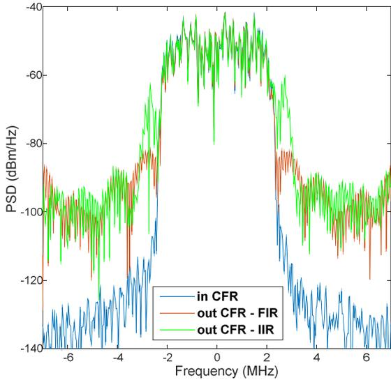
Fig. 3. Power spectral densities at CFR input and output.
