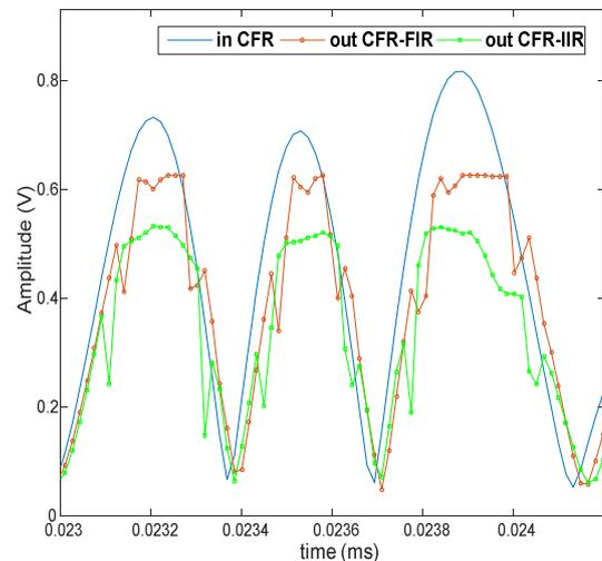
Fig. 2. Amplitude waveforms at CFR input and output.
