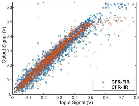
Fig. 4. CFR output amplitude in function of CFR input amplitude, for FIR and IIR filters.
