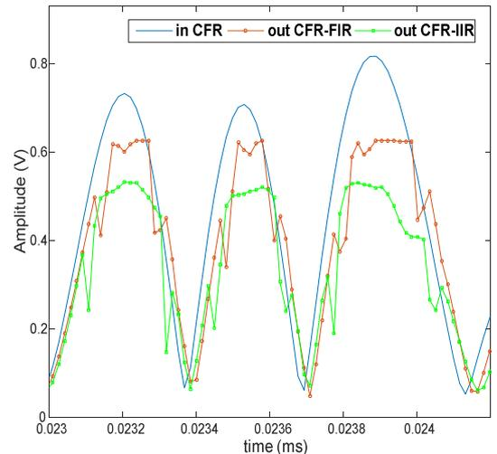
Fig. 2. Amplitude waveforms at CFR input and output.
