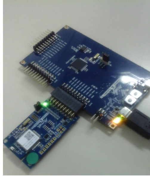
Fig. 4. SAMD21 with the ATBTLC1000 peripheral connected to a computer.
