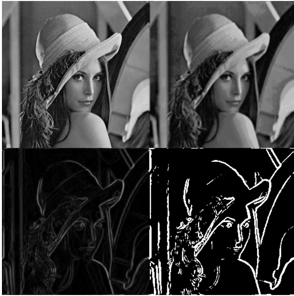
Fig. 6. Input image, the image after the sobel method and after the threshold apply
