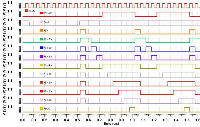
Fig. 3. Control logic signals for a constant input signal of 123.45 mV.
