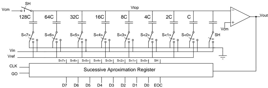
Fig. 1. Simplified schematic diagram of a 8-bit SAR ADC.
