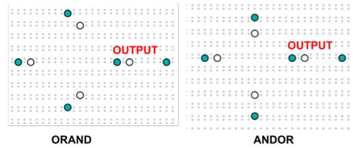
Fig. 2. SQD-based 3-input gates. (a) ORAND. (b) ANDOR.
