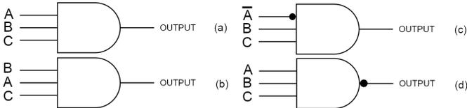
Fig. 1. Configurations from a same NPN class. (a) Original AND gate. (b) inputs permutation. (c) input A complement. (d) output complement.
