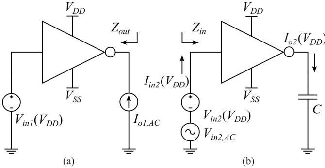
Fig. 2. Schematic circuits of the ring oscillator test bench: (a) output impedance; (b) both transconductance and input capacitance.
