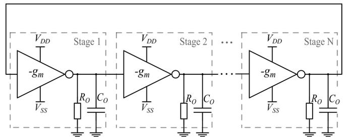
Fig. 1. Schematic circuit of the  $N$ -stages Ring Oscillator (RO).
