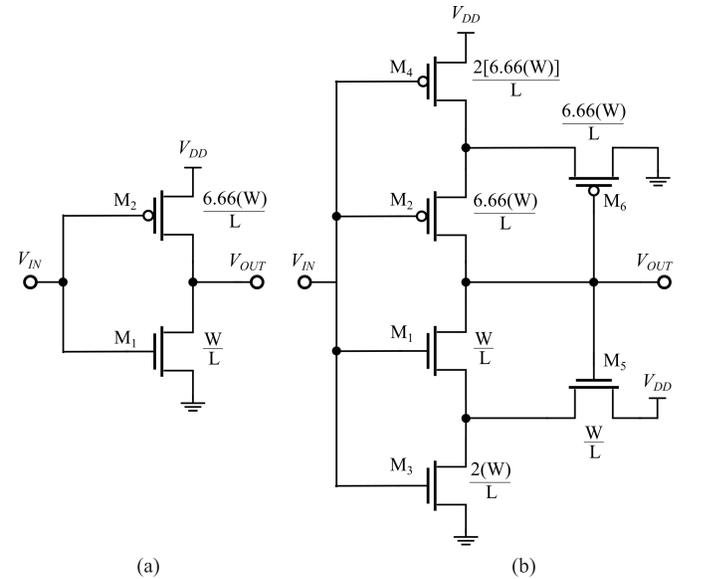
Fig. 3. Schematic circuits of characterized inverters: (a) traditional (INV); (b) Schmitt Trigger (ST).
