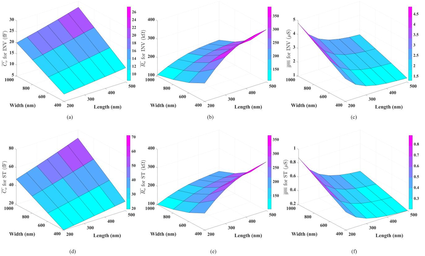
Fig. 4. Average values of output capacitance, output resistance and transconductance for inverters INV and ST, which were computed from Eqs. (9), (10) and (11), respectively.
